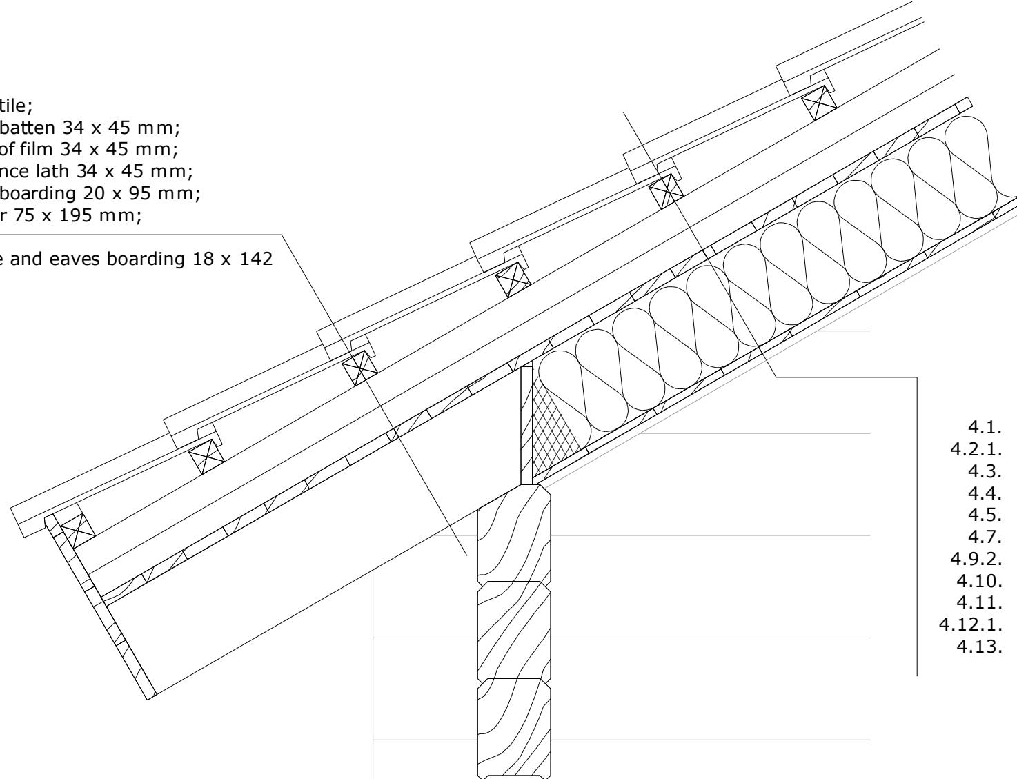
In case of ceramic rooftile the minimum roof angle is 22 degrees and in case of cement rooftile it is 14 degrees
